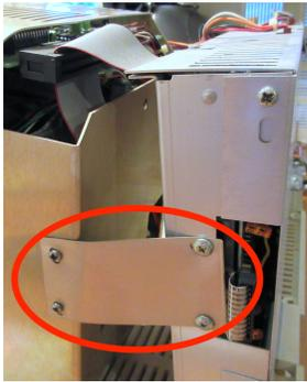
Step 1: Remove the protective ribbon cable bracket.
