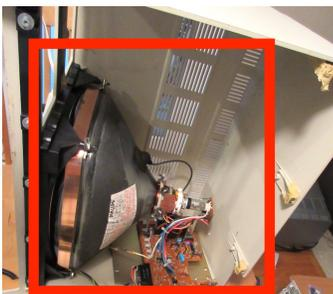
**NOTE:** Avoid making contact with the monitor tube and related circuit board as they contain very **High Voltage**.
