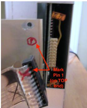
Step 2: Mark the TOP edge of your existing keyboard cable as "Pin 1". Then gently unplug your existing keyboard ribbon cable from the TRS-80 motherboard connector.
