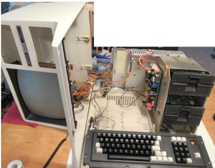
Step 3: Carefully lift the case **STRAIGHT UP**. There is a fragile neck on the back of the monitor tube that can be easily damaged. Lifting the case straight up will prevent damage. You can look into the top of the vents above the rear of the monitor tube to see the neck and watch it for clearance as you lift.
