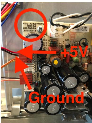
The included wire crimp connectors are easy to use. Just cut an existing +5V (red) power wire (with the TRS-80 TURNED OFF). Then insert the two ends of the wire into the crimp connector along with the related NEWKEY/80 power cable wire (+5 or ground). Crimp the three ends together with a pair of pliers. Try to crimp straight down, not at an angle. Repeat for the ground (black) wire.
