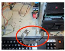
Step 3: Gently feed your existing keyboard cable under the drives (if present) and into the empty space in front of the keyboard.
