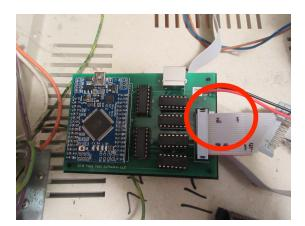
Step 5: Plug the other end of the NEWKEY/80 ribbon cable into the NEWKEY/80 adapter, aligning Pin 1 markings.
