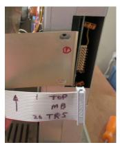
Step 4: Plug the NEWKEY/80 ribbon cable (marked "TRS") into TRS-80 motherboard connector with Pin 1 at the TOP and re-attach the protective metal keyboard cable bracket.
