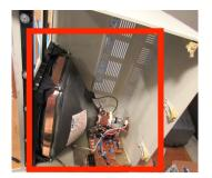
**NOTE:** Avoid making contact with the monitor tube and related circuit board as they contain very **High Voltage**.
