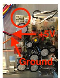
The included wire crimp connectors are easy to use. Just cut an existing +5V (red) power wire (with the TRS-80 TURNED OFF). Then insert the two ends of the wire into the crimp connector along with the related NEWKEY/80 power cable wire (+5 or ground). Crimp the three ends together with a pair of pliers. Try to crimp straight down, not at an angle. Repeat for the ground (black) wire.
