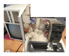
Step 3: Carefully lift the case **STRAIGHT UP**. There is a fragile neck on the back of the monitor tube that can be easily damaged. Lifting the case straight up will prevent damage. You can look into the top of the vents above the rear of the monitor tube to see the neck and watch it for clearance as you lift.
