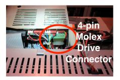
**For a Disk-Based TRS-80**, the easiest method is to use the included Molex 4-Pin disk drive Y-Splitter cable.
