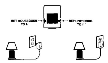
Press the top "1" button (for unit code 1) on the Controller and the lamp will go on. Press the bottom "1" button (for unit code 1) and the lamp will go off. Refer to Appendix B, Troubleshooting, if this does not happen.
